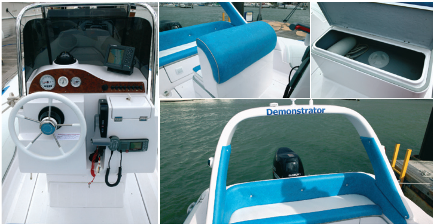
Pictures clockwise: Console, seating, storage compartments and fibreglass 'A' frame - perfect for arials and other antennae.
